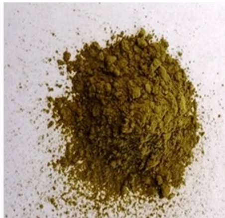
Figure 5 – Flotation-enriched glauconite concentrate of «Changi» deposit
