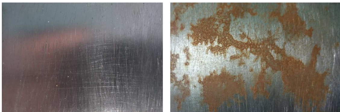
Fig.1. The effect of IK-2 (a) and Incorgaz T 21 (b) on the metal St-20 at 30–60 °C
