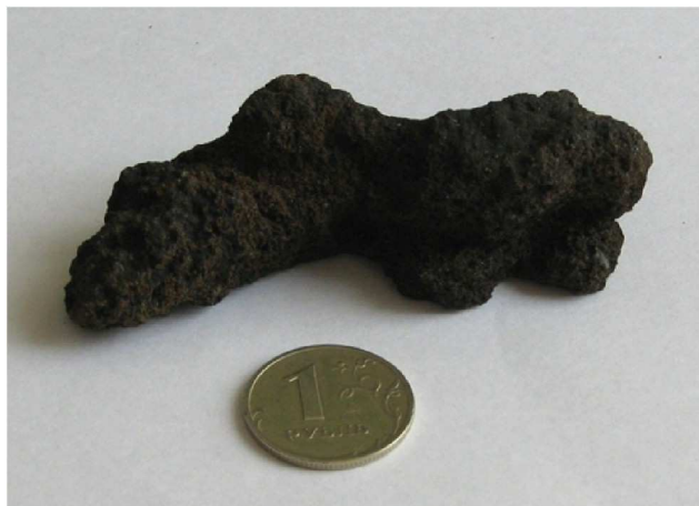
Figure 10 – Fragment of scale which was removed from power cylinder bush. Diameter of the coin is 19.45 mm
